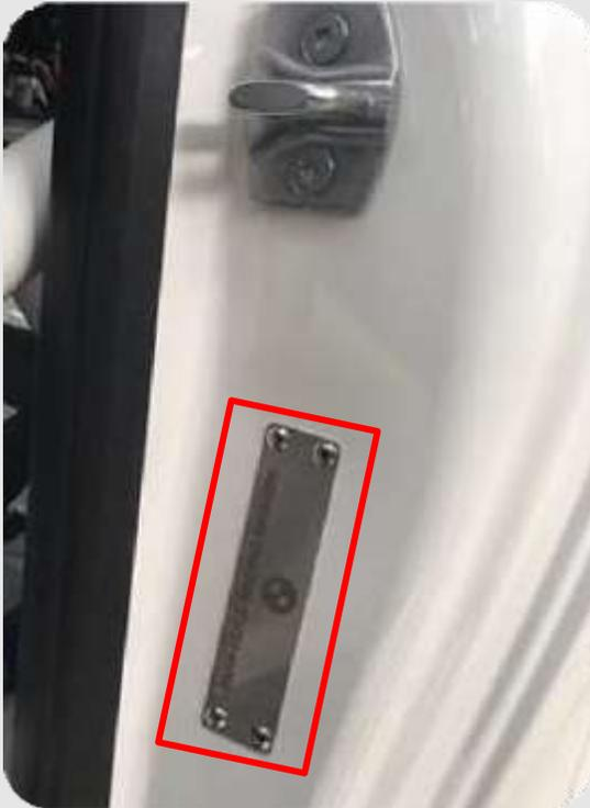
The Chassis-No. (e.g. 1901) is located at the B-Pillar on the driver side entry.
