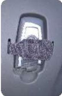
The ID transmitter (remote control) must be present for starting the engine in the vehicle. The position shown in the center console is provided for this purpose.
