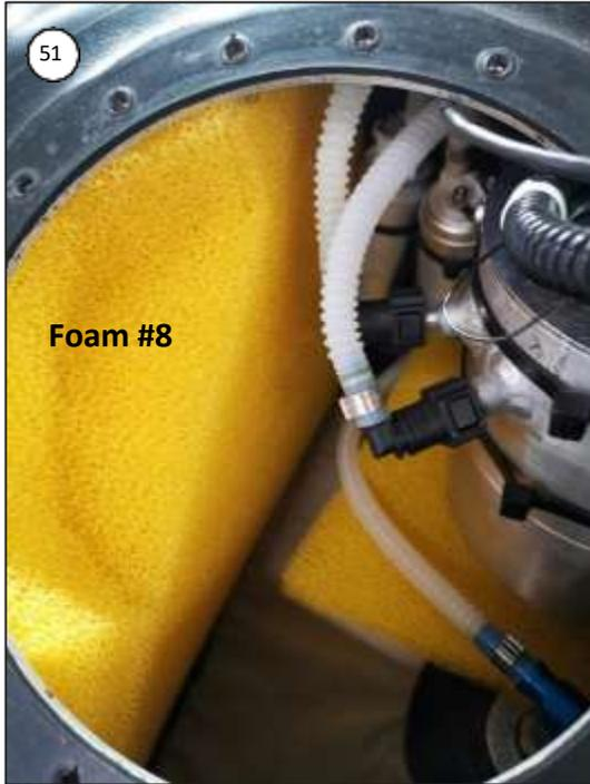
Take foam #8, that you left aside during the dismantling phase (Picture #19) and place it through the opening inside the tank on the very far left side.
