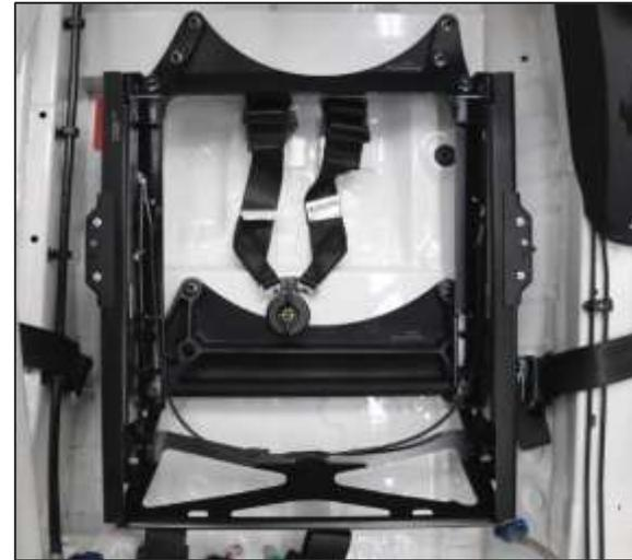
5. Only then remove the transport lock. The remaining screws should be kept at later for fitting the seat to the console.
