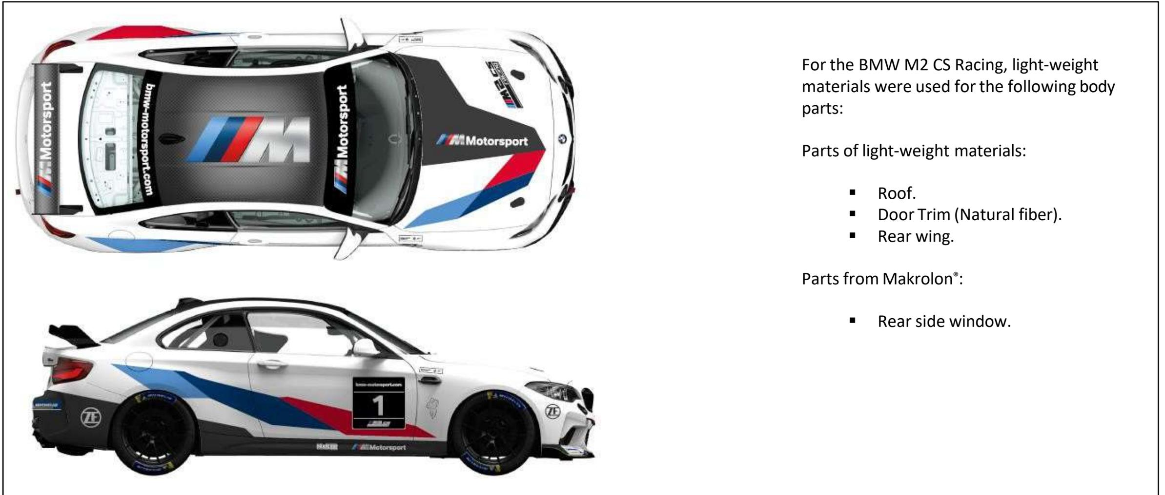
For the BMW M2 CS Racing, light-weight materials were used for the following body parts:
