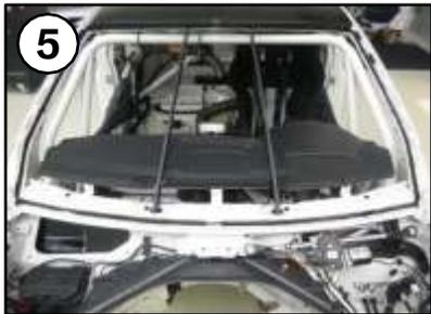
Analog fit the front support struts, treat the adhesive surface and add the Würth Ultimate around the windscreen flange.
