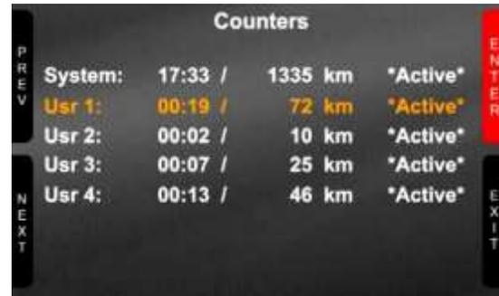
To reset the odometer scroll to "Clear" option to one of the labelled "Usr" and press "ENTER", the odometer resets for that "Usr".
