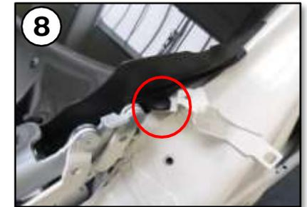
Fit windshield with 2x plastic clips to body bracket (fender) L / R.
