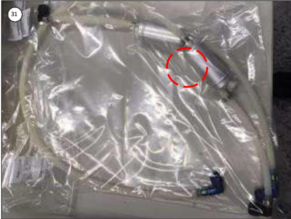
Take the two lift pumps (picture above) and the 4 cable ties (4,8x280mm) PN 8342900-001-A (Item #9 on picture #20).
