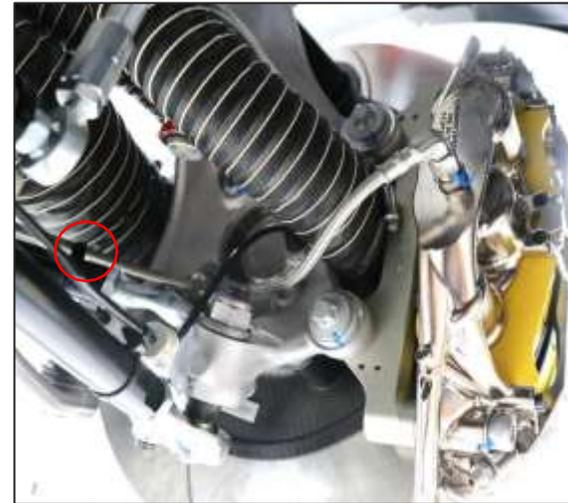
12. Connect brake line as shown with an angle of approx. 45 ° and fasten it with double head cable ties.
