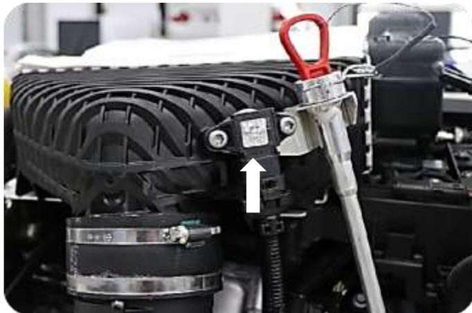
P/T-Sensor Intercooler (1x Hologram)
