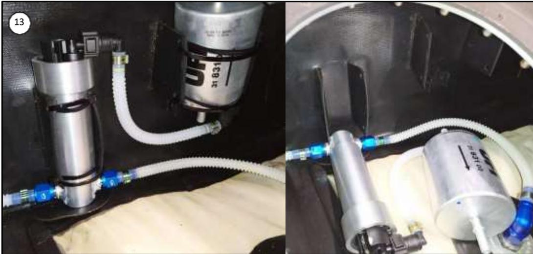
By the use of a cutter, remove the cable ties, that hold these two parts (5 pieces in total, two on the pump, and 3 on the filter – two big and a little one on the bottom).
