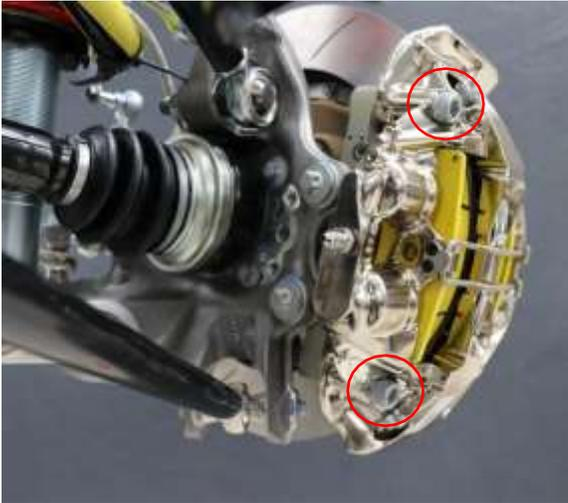
8. Mount the caliper on the adapter as shown. The screw connection is made **without** a washer.
