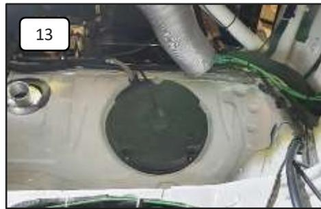
Apply fuel line to fuel tank mount (service cover) and attach service cap with plug to it and fasten. Screw the firewall including the seal back onto the floor panel.
