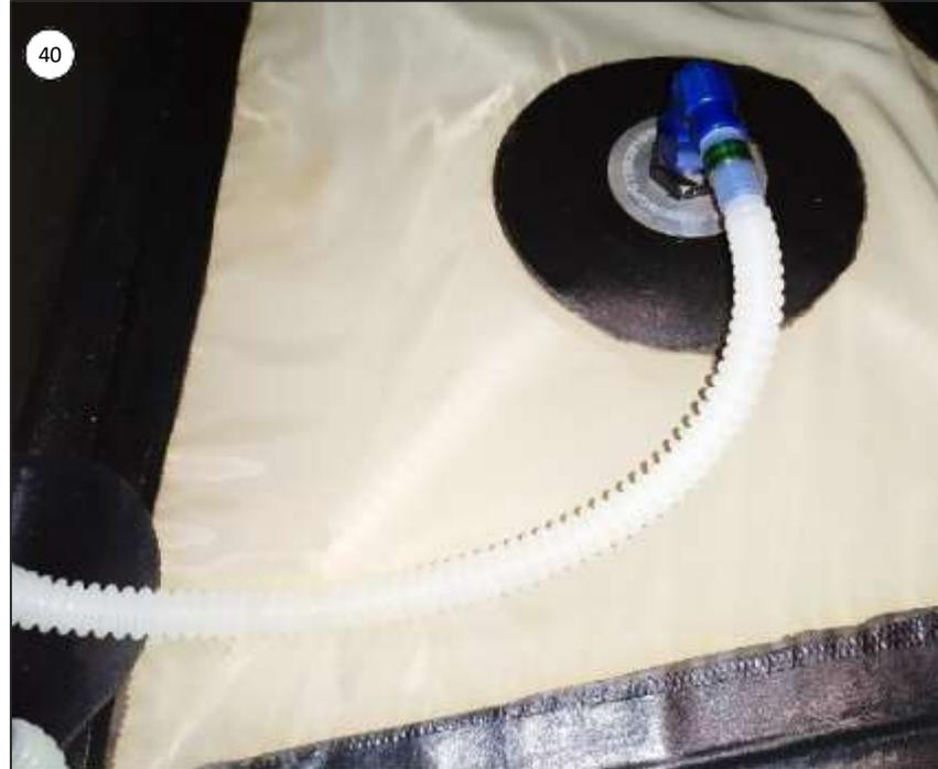
Slightly unscrew the Goodridge fitting and turn it of about 90° together with the hose. Then tight it again with 22-26 Nm.
