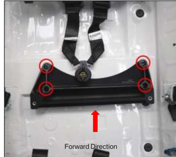
3. Mount the seat adapter at the rear as shown with bolt and washer.
