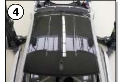
Insert, position and fix the CFK Roof carefully onto the body.
