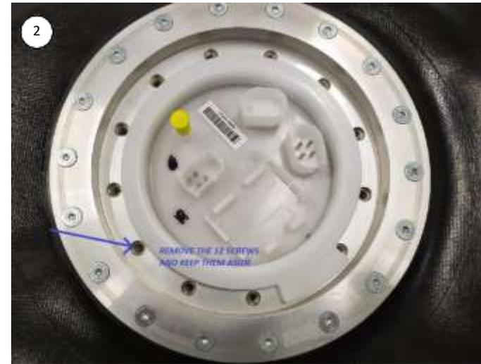
Remove the inner 12 screws, carefully from the internal metal ring of the fuel pump and **put them aside for later.**
