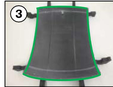
Put Würth Ultimate adhesive with a 2K dispensing gun to the marked roof flange of the body (green).
