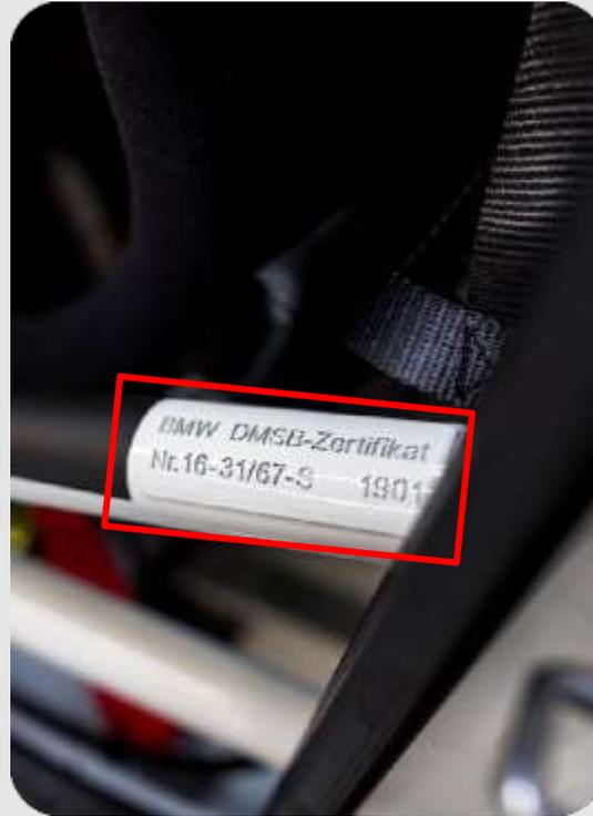
The Cage-No. (e.g. 16-31/67-S) and the Chassis-No. (e.g. 1901) are located on the driver side near the B-pillar on the cage tube.
