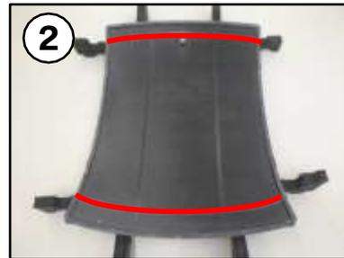
Put window adhesive front and rear of the roof bend inside the marked areas (red) on the body.
