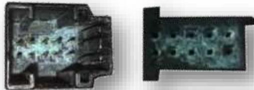
If corrosion is present, then clean and dry the plug as best as possible using suitable means (e.g. contact spray).
