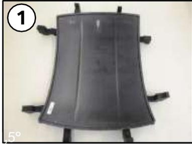
Treat the adhesive surfaces on carbon roof and body with abrasive fleece and clean it with cleaner R1.
