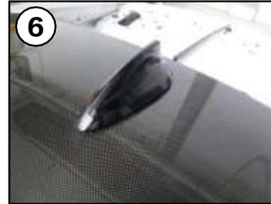
Put the roof antenna including GPS receiver into the CFK Roof from above.
