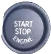
When the start / stop button is pressed and the brake is actuated at the same time, the engine starts in each terminal state. If only the Start / Stop button is pressed without the brakes, the ignition can be switched on or off.
