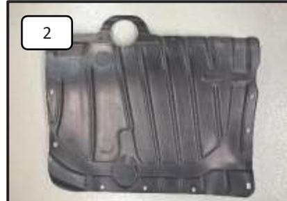
Use the cover plate (P/N 8342796) as a template to set the drill holes only.
