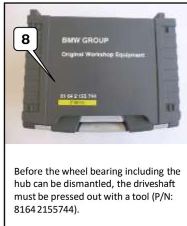
Before the wheel bearing including the hub can be dismantled, the driveshaft must be pressed out with a tool (P/N: 8164 2155744).
