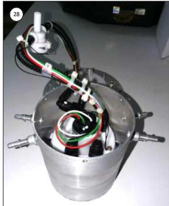
Take the pump body and insert it inside the catch tank pushing it down until it is perfectly matching with the metal ring inside. Pay attention to the catch tank orientation. Catch tank, pump and hex screws orientation must be as shown on the below picture.
