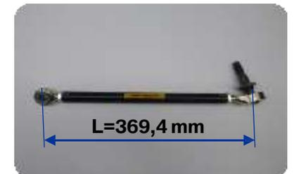
For this purpose, a suspension strut adjustment gauge from BMW M Motorsport is offered:
