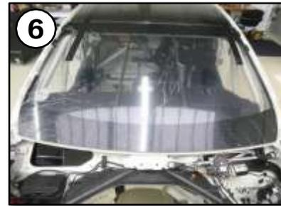
Insert, position and fix the windscreen carefully onto the body. Connect the front screen heating cable harness to the windscreen connector.
