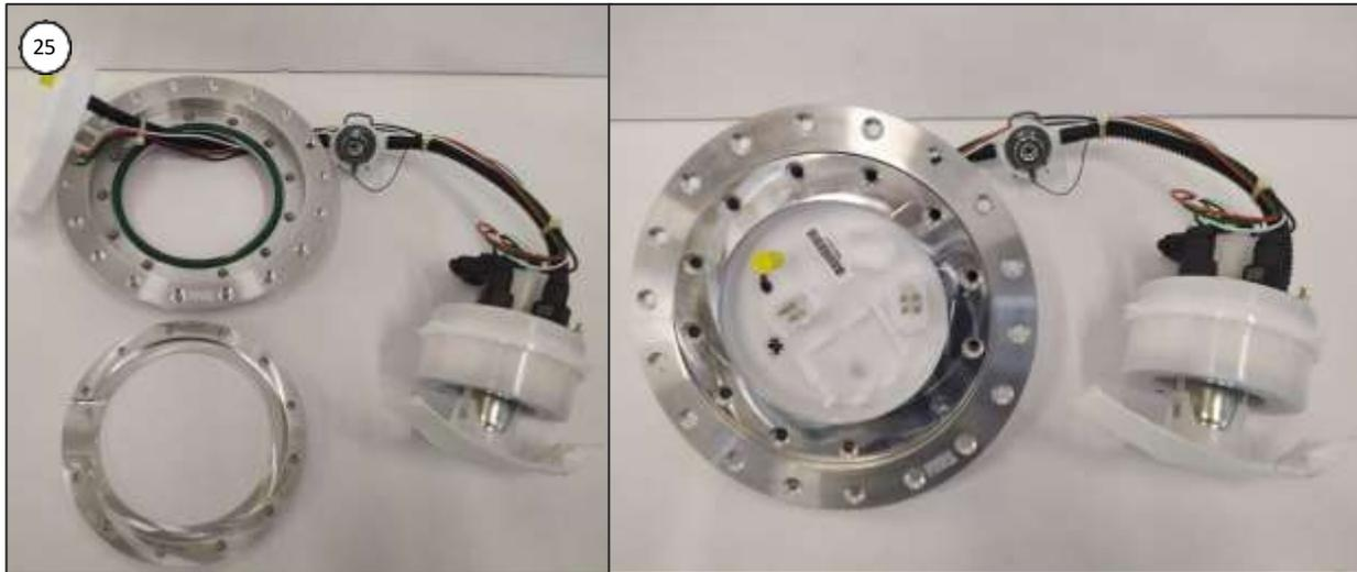
Place the O-ring inside it's seat (left picture) and close it with the inner flange on top (right picture).
