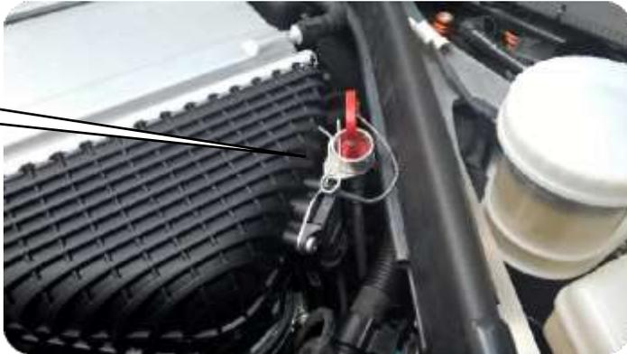
**Min:** 6.8 L (with Filter)    **Max:** 8.4 L (with Filter)
