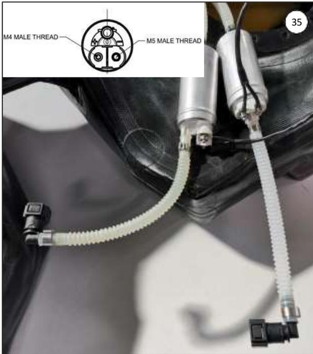
Then, take the electrical loom received with the KIT, see picture #20 (item #13), and install it, see picture above.
