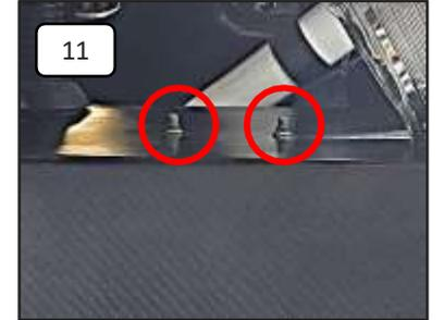
Screw the tank bladder to the firewall with a third person from above.
