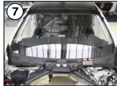
Lock windshield with 9x plastic hexagon quick-release fastener on windscreen.
