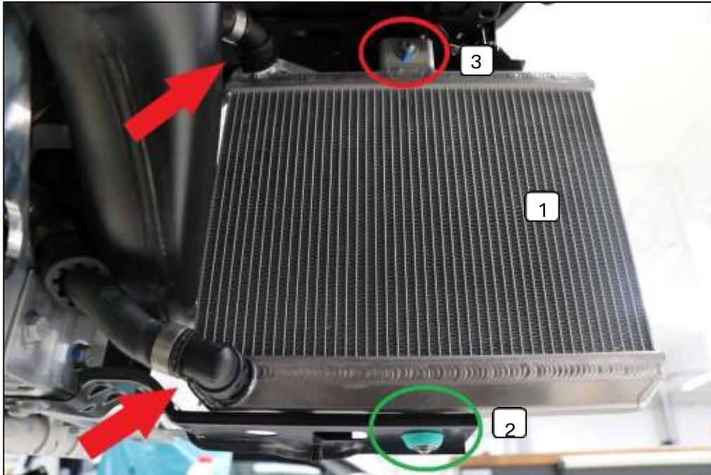
9. Insert the new coolant radiator (1) into the rubber mount (2) and secure it with the screw M5 + washer as shown.
