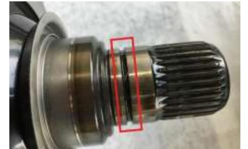
6. Insert driveshaft again with a new safety clip and assemble in vice versa sequence.
