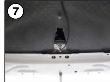
Fix the roof antenna with 3x Kaynut M5 from inside.
