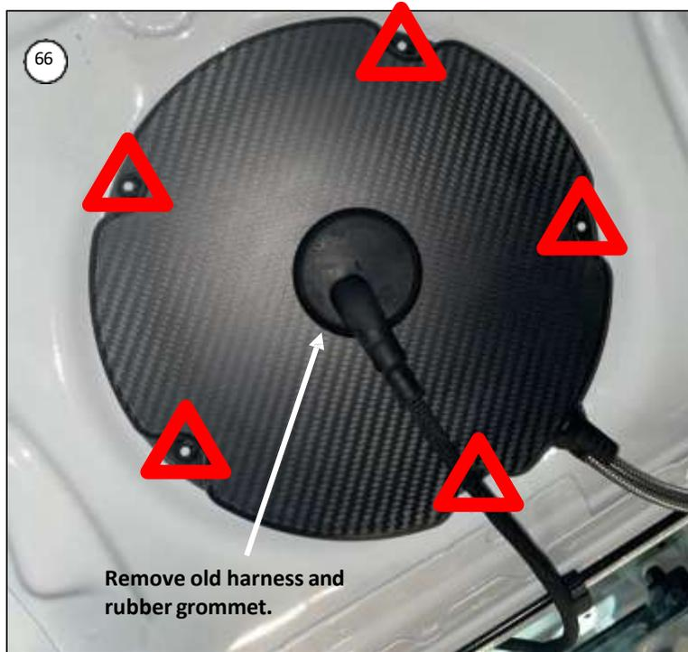
First remove the five plastic nuts (red triangles) from the carbon fuel pump cover and remove the cover.
