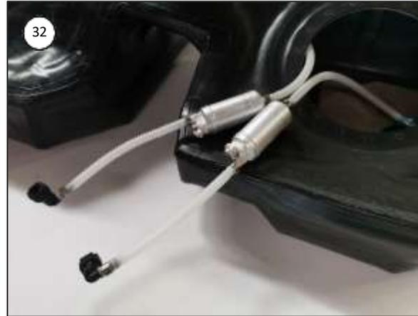
Connect the two lift pumps with the D06 connector to the pickup points.
