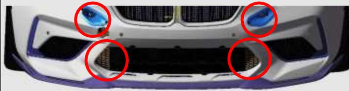
To achieve the optimum brake disc temperatures, the blanking of only the lower ducts should be done on the 365 BHP version due to caliper cooling by the upper ducts.
