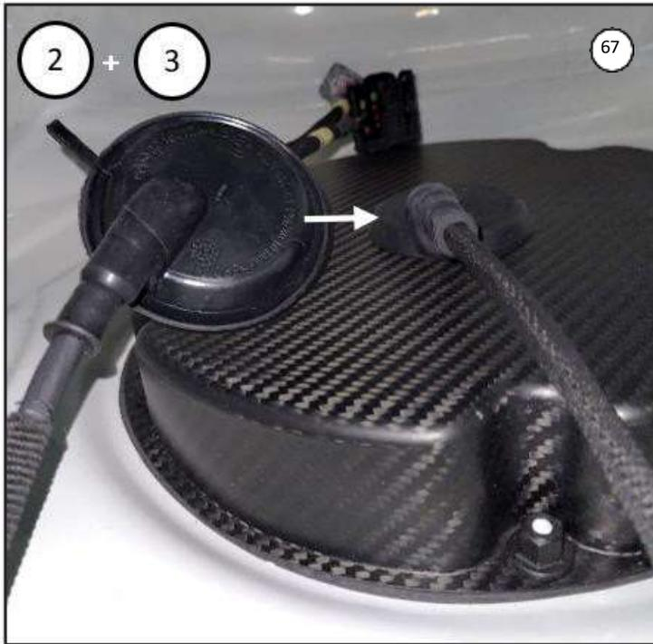
Route the two connectors (2+3) from the new harness including the rubber grommet, through the middle hole of the carbon cover and connect the connectors to the fuel pump. Make sure the rubber grommet fits correctly.
