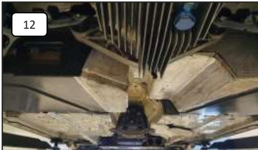
Screw the tank pan with 6x bolts M8x20 to the body.
