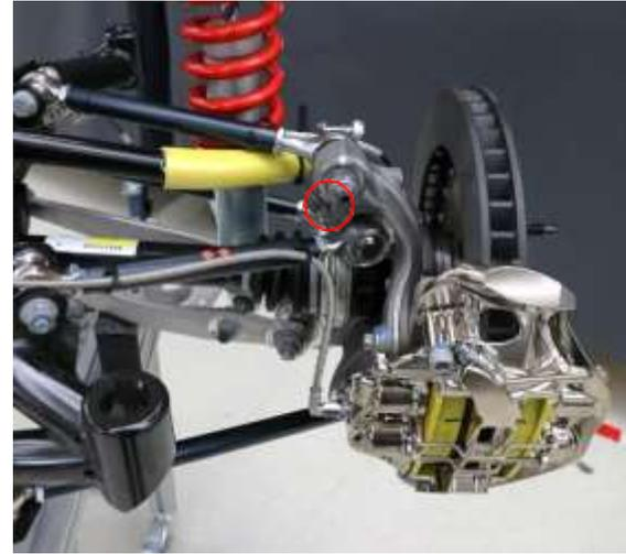
9. Connect the brake line as shown and secure with a double-headed cable tie.
