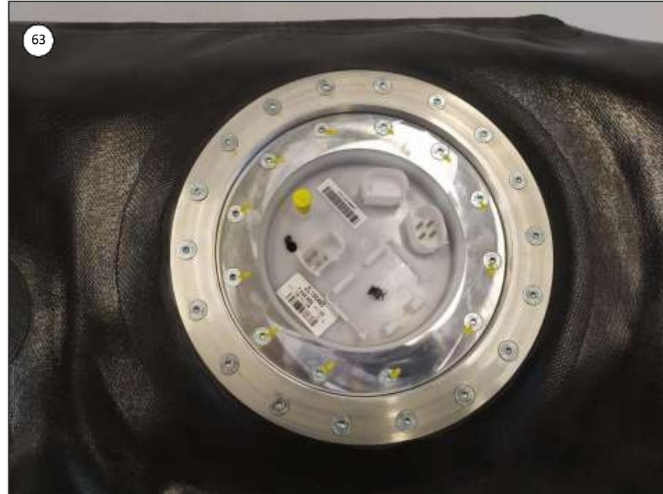
Close the flange opening with the already assembled closure plate and tight the remaining 18 screws with 6-8 Nm. See picture above.
