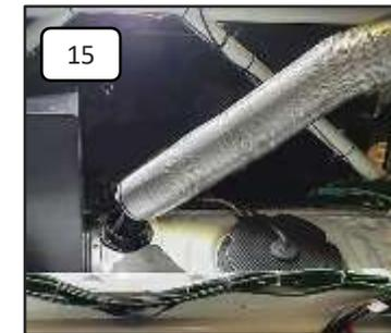
Fit fuel filler hose to tank with hose clamp. Fasten aluminum protective hose with clamp.
