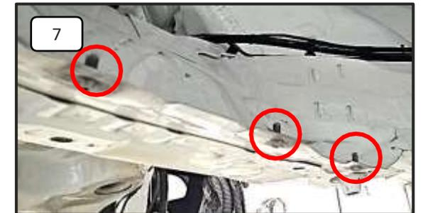
Insert the fillister head screws M5x12 (P/N 8435913) from below through all holes and spot-weld them on as shown. Before doing this, sand down the contact surfaces and flatten the weld area. After, paint the sanded surfaces again and mask the screw heads with helitape.
