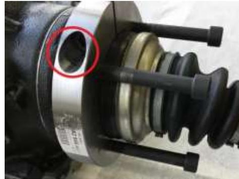
3. Turn the driveshafts until the screws 8427181 are aligned with the screws of the diff cover.
