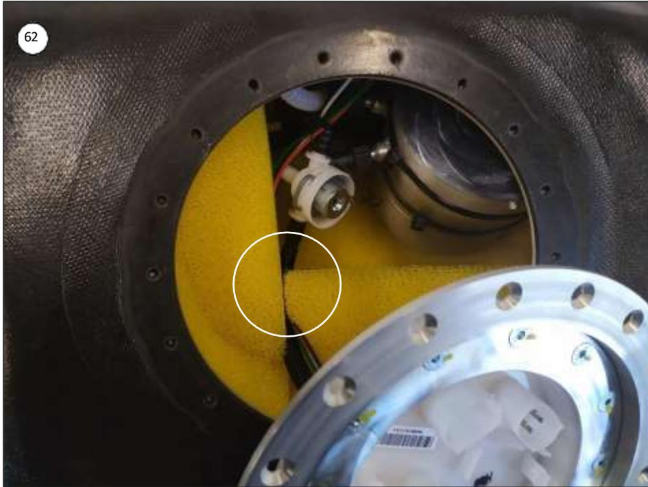
Arrange/route the HP hose with the cables to pass between the piece of foam #8 and #10. See picture above.
