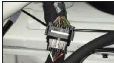
Disconnect this plug if pumps need to be switched off, while ignition is on.
