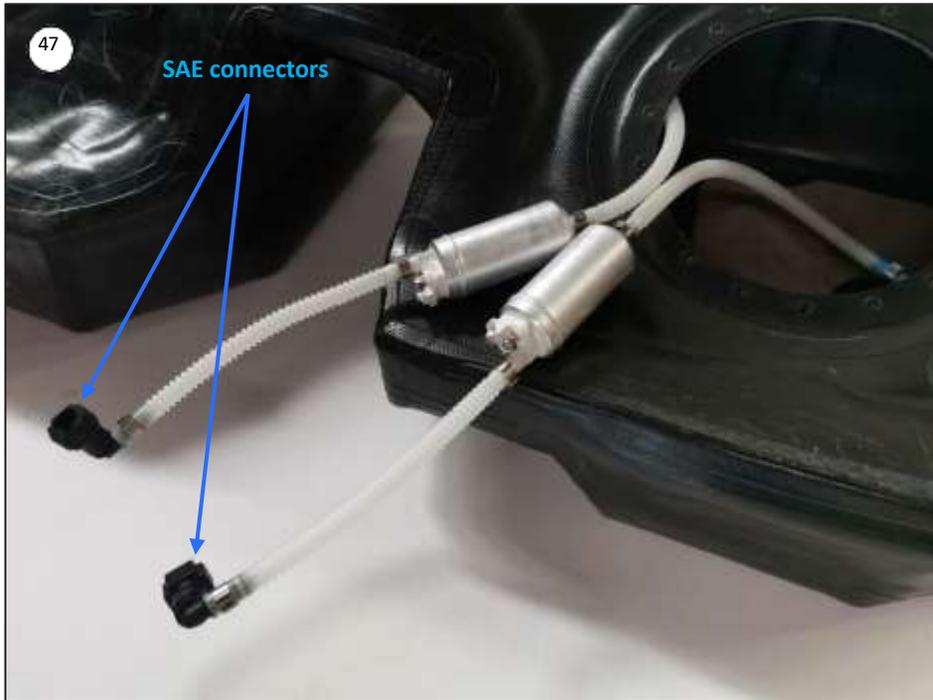
The free SAE connectors at the end of each lift pump hose, must be now connected to the catch tank hose holders.
