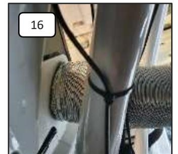
Attach fuel filler hose and aluminum protective hose analog to the tank filler neck.
