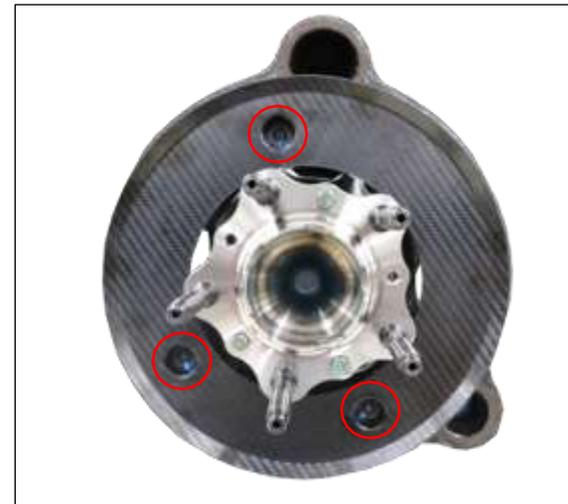
3. Fit the brake air duct cover disc as shown.
