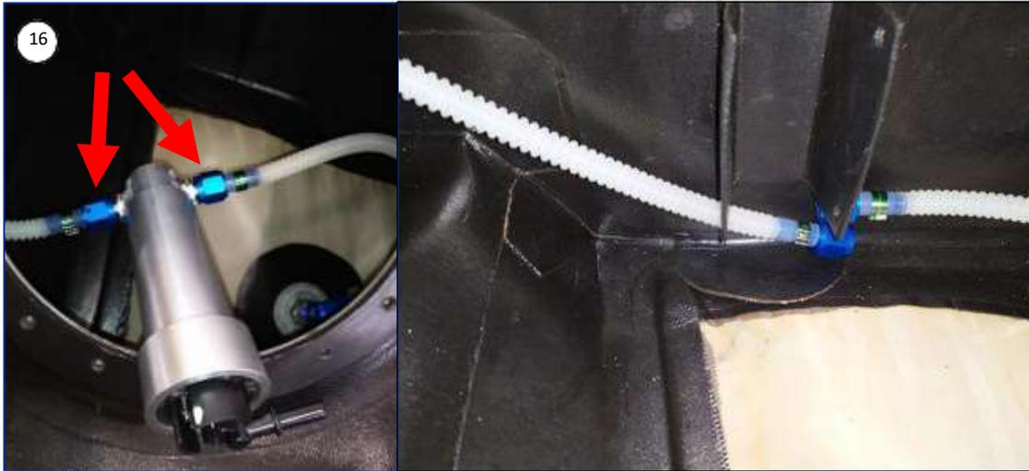
Now, unscrew the two blue connectors, screwed on the fuel pump support (D06) on the bottom. Then leave the hoses inside the tank.
