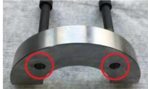
3. Attach the tool to the driveshaft as shown and screw together with 8427901 (20 Nm).
