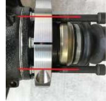
4. Tighten screws crosswise in 10 Nm steps with a torque wrench until driveshaft "pops out".
