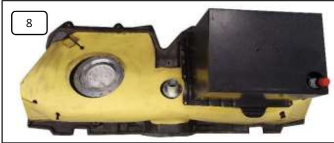
Prepare tank bladder with CFK firewall, tank protection (Sylomer) and tank pan. Sprinkle the tank tray with talcum powder beforehand.
