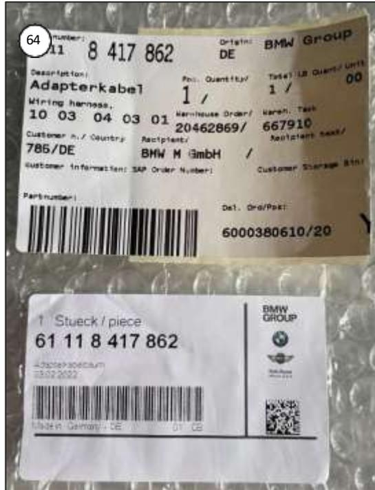
Verify that you received the right parts by part number and check the harness including the pins for any damage.
