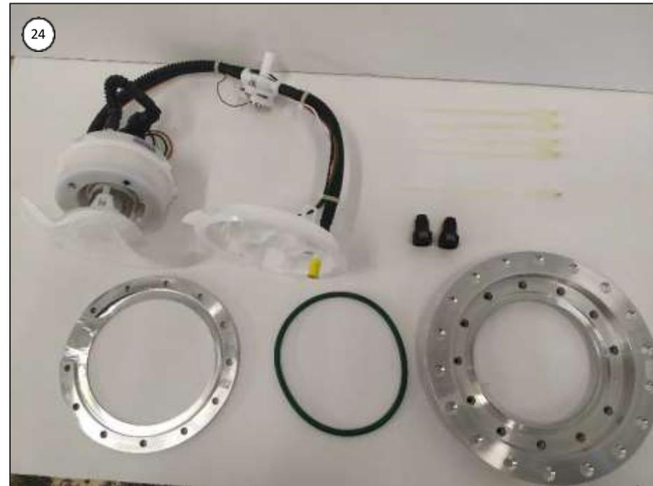
Above you can see the needed parts to start assembling the OEM-Pump and its supporting metallic flange.
