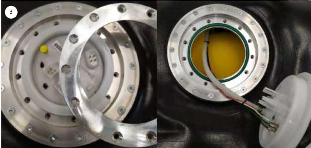
Soon after removing the metallic flange (left picture), raise the plastic plate (right picture) and follow the corrugated hose until to the connection with the UFI filter. Then disconnect the hose from the filter, using the SAE quick connector's push-button and remove the green O-ring (see picture far right).
