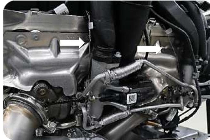
Turbocharger Bank 1 + 2 (2x Cable Seal)
