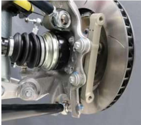
5. Fit brake caliper adapter to wheel carrier as shown. Observe the notes below.
