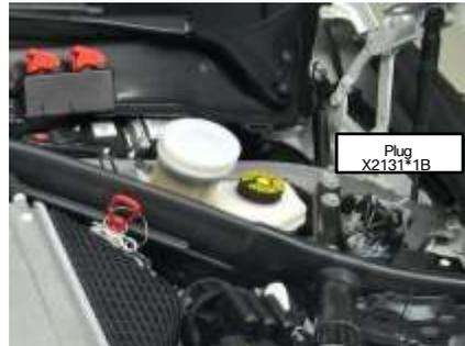
Open plug connection and check both sides (male / female) for corrosion.
