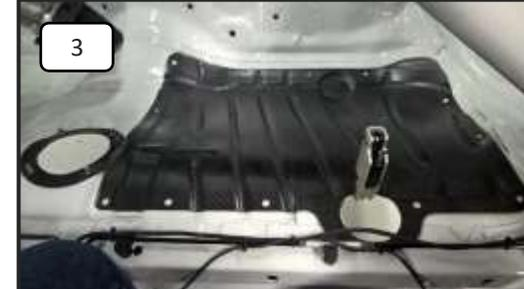
Align the template (cover plate) and fix it with a clamp.
