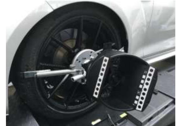
Remove the guide pin from the adapter at this position if the pin can touch the screw as shown.
