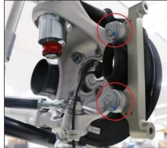
8. Fit brake caliper adapter to wheel carrier as shown. Observe the note below.
