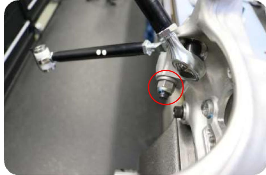
Screw the suspension arm to the wheel carrier (rear position).
