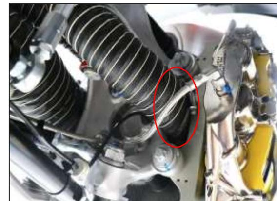
4. After, fit the brake air hoses. Note that the brake air hose of the brake caliper cooling (365 HP) is inserted on the opening (1) in the new brake air duct. Regarding laying and, if necessary, length compensation, it is recommended to slide the brake hose a little forward into the cooling module and to be reattached with double head cable ties.
