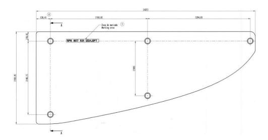
The foremost edge of the front splitter at y=0 will protrude the bumper contour by max. 35mm in vertical projection.
